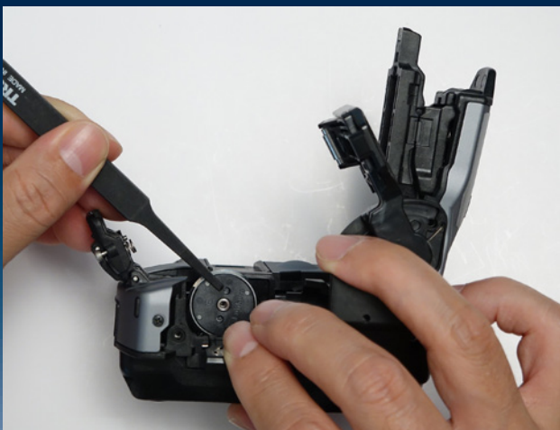
User replaceable cleaver blade
