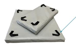
Sewn nylon loops provided to secure RF panels while testing
