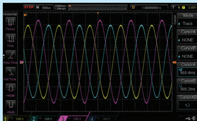
Three Phase Unbalance Voltage Test Captured
