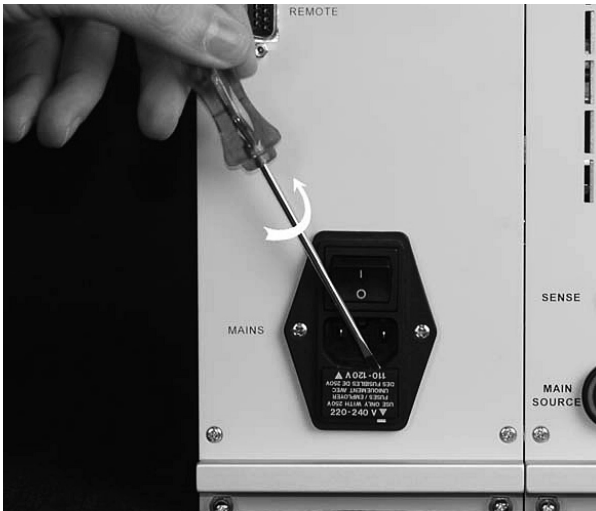
Picture 2-2: Loosen the drawer using a screwdriver
