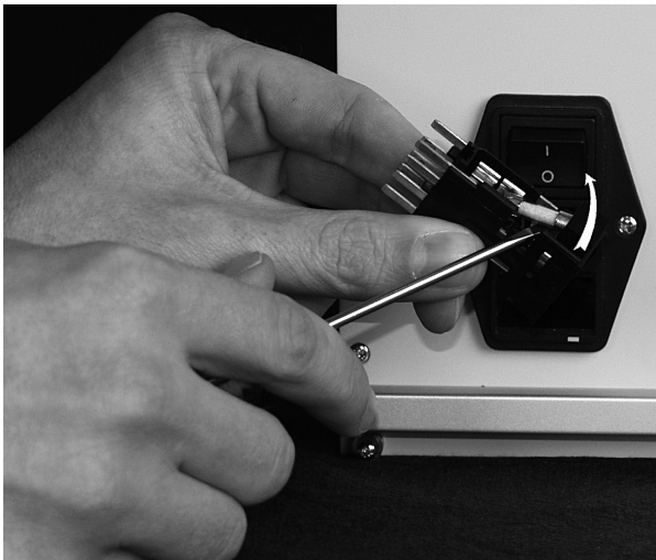
Picture 4-5: Remove defect fuses.
