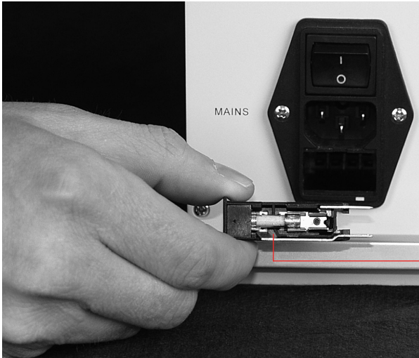
Picture 4-4: The Fuses are placed on the sides of the drawer.
