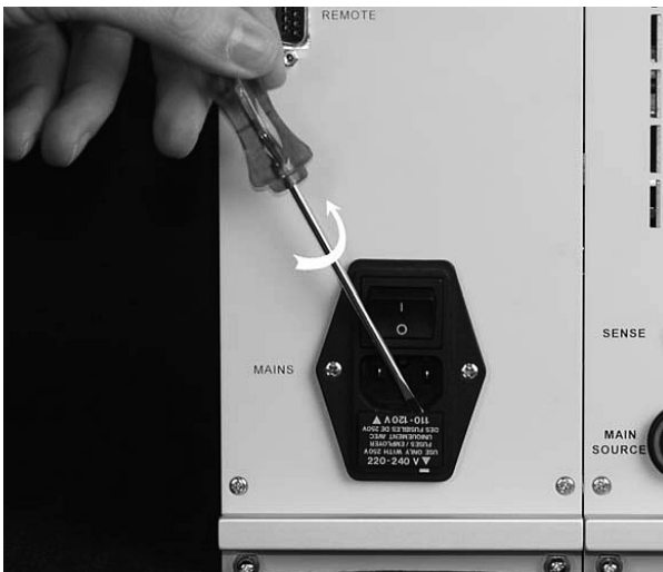
Picture 4-2: Loosen the drawer using a screwdriver.
