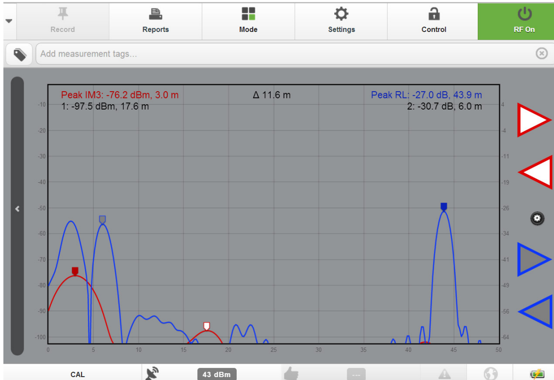
Figure 38 Range to Fault (RTF) Measurement Window
