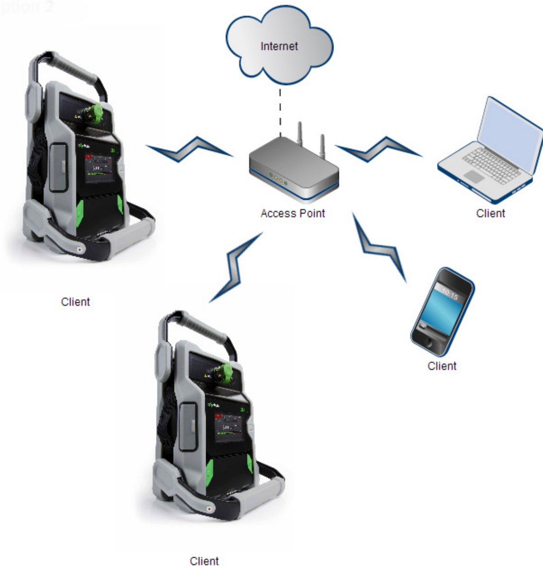
Figure 60 Wi-Fi Connection Options (external access point)
