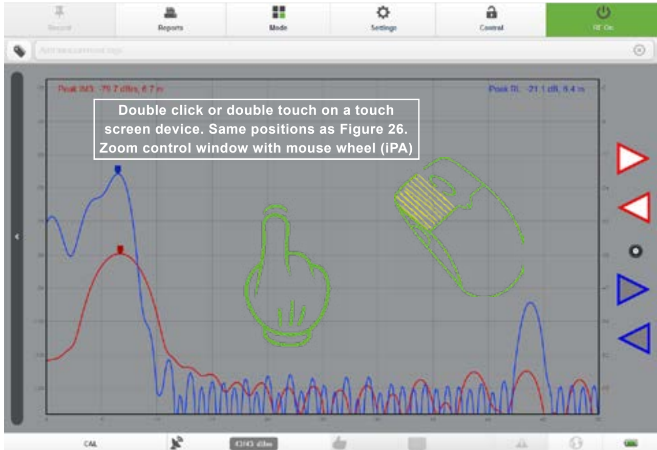
Figure 27 Zoom control window with duoble mouse click or touch pad (iPA Remote PC Screen)
