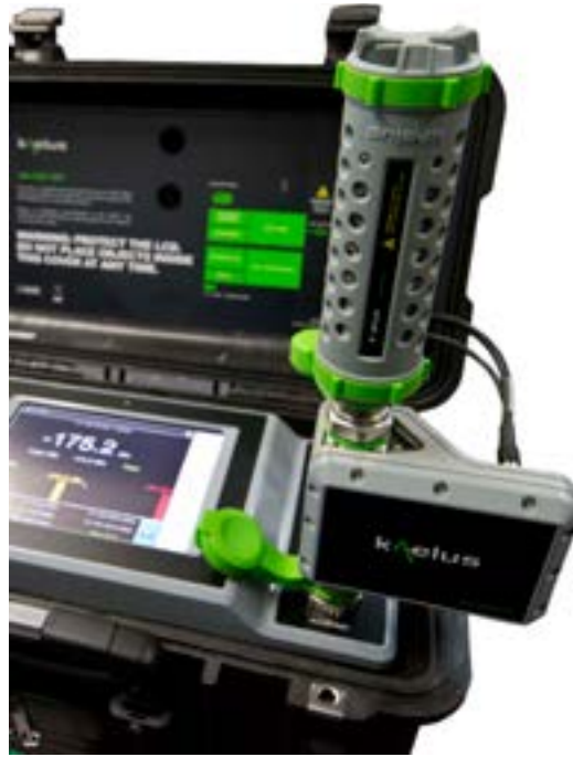
Figure 6 RTF module on the iQA (CIS-0001A PIM Source used for 5th order calibration)
