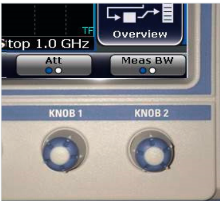
Two rotary knobs with user-assignable functions.
