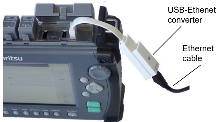
Figure 11.2.1-1 Ethernet Cable Connection
