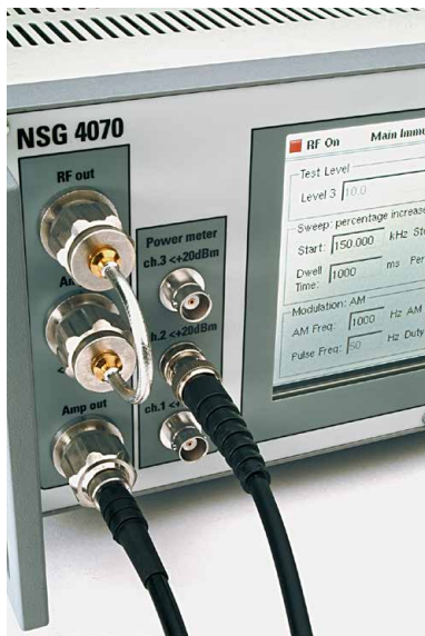
NSG 4070 front panel with RF ports
