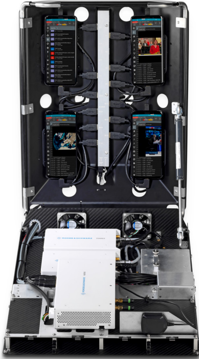
R&S®FR4-CORE with mounted mobile phones and scanner.
