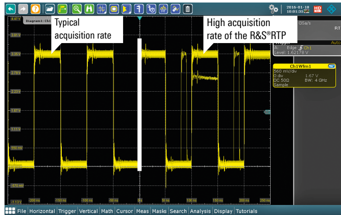
The high acquisition rate detects sporadic signal faults fast
