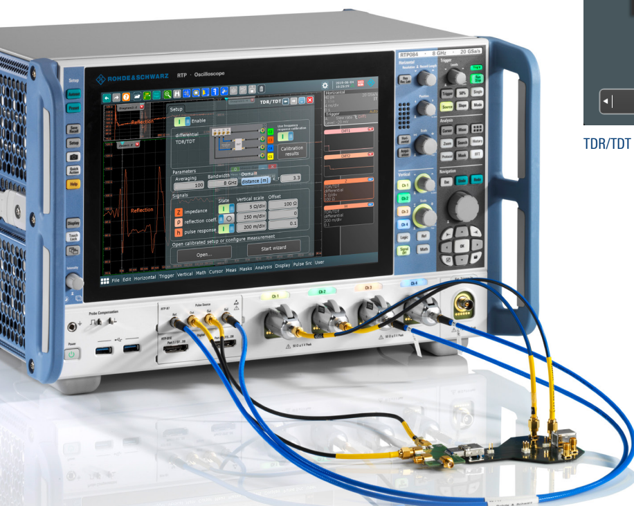
Differential test setup with the R&S®RTP-B7 pulse source and the R&S®RTP-K130 TDR/TDT analysis option
