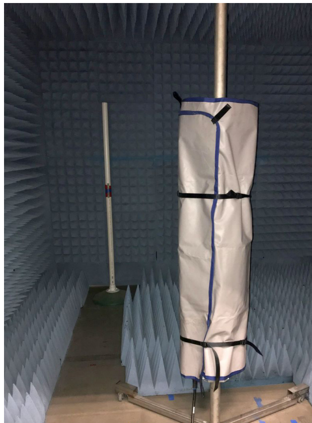
Antenna Wrapped in PIM Blanket
