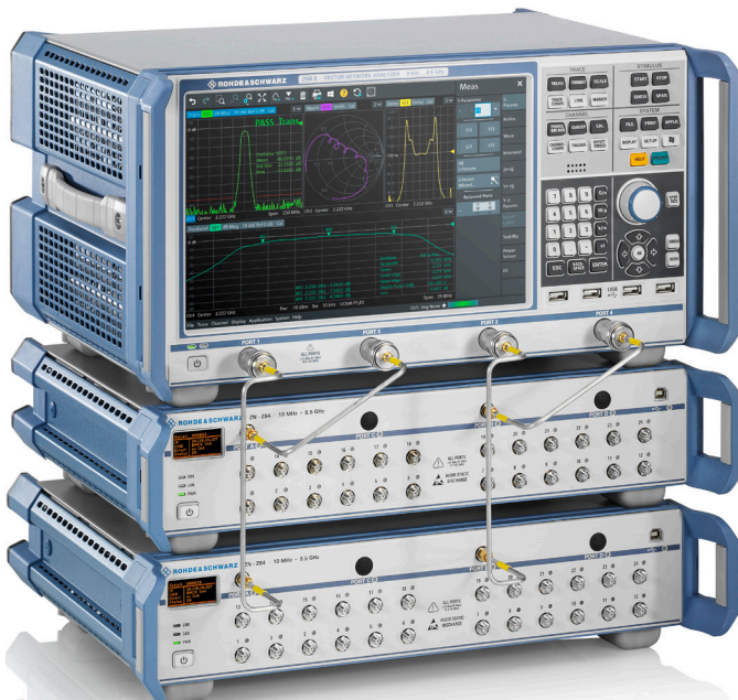
R&S®ZNB with two R&S®ZN-Z84 switch matrices
