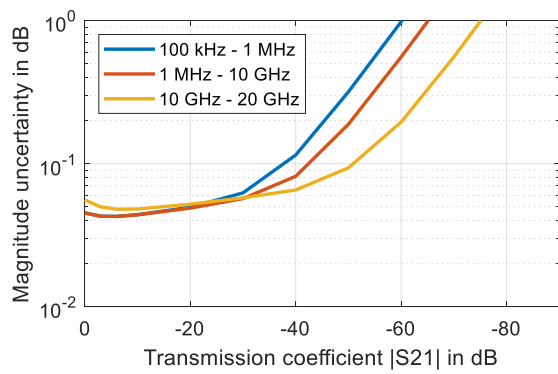
Typical uncertainty of transmission magnitude and transmission phase measurements for the R&S®ZNB20 in the frequency range from 100 kHz to 20 GHz; Analysis conditions: S_{11} = S_{22} = 0 , cal. power –10 dBm, meas. power –10 dBm
