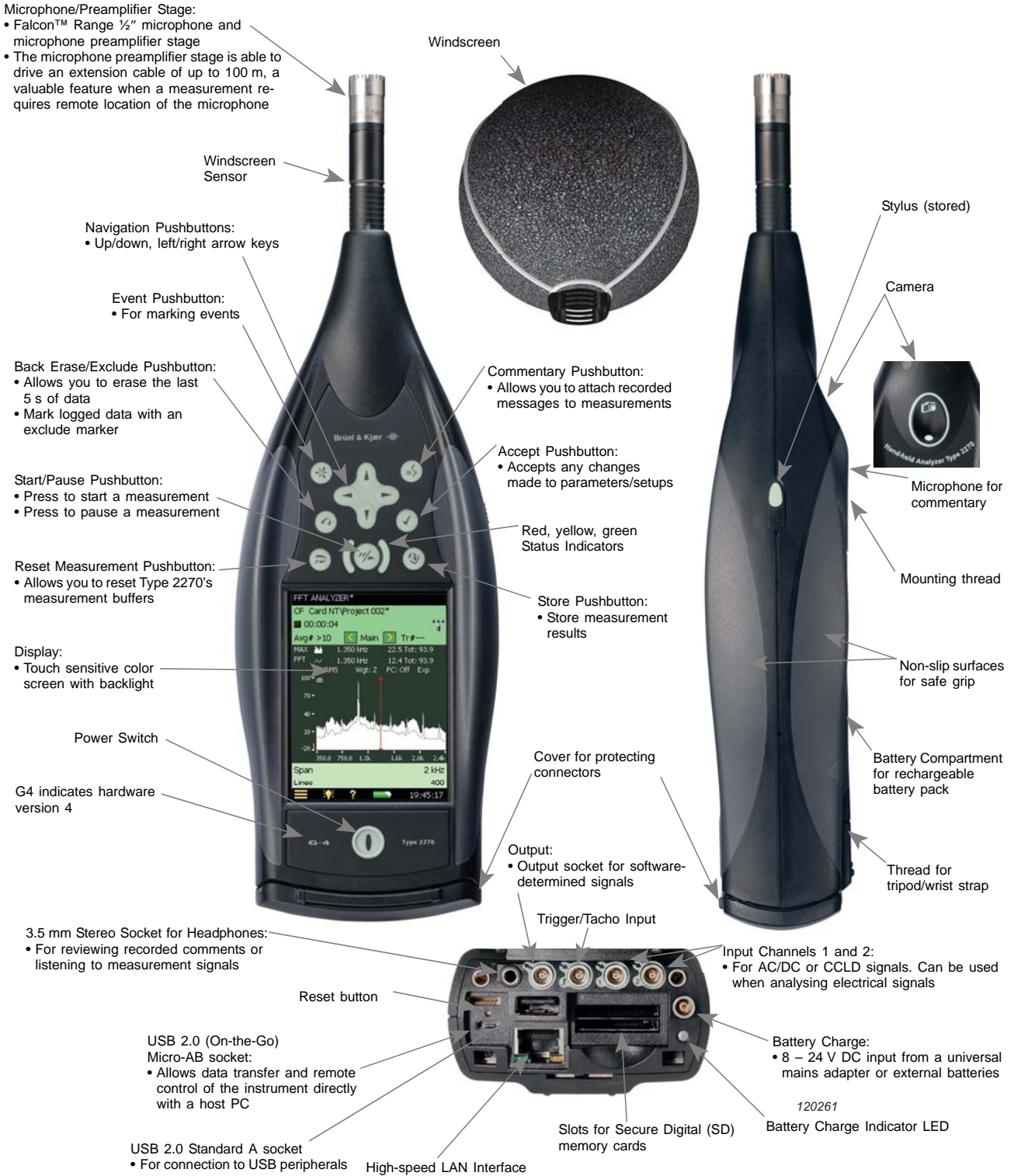
Fig. 3 Key features of Hand-held Analyzer Type 2270
