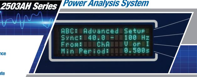
The 2503AH Analyzers measure power, voltage, and current up to 500 kHz with premier precision. Available parameters include V, A, W, Power Factor, Crest Factor, K Factor, THD, Harmonics, Phase, VA, VAR, W.Hr, Triplens, Impedance, Inrush, Mean-Peak Values, Efficiency-Loss, etc.
