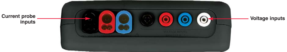
The color-coded input connectors provide dedicated current probe inputs and voltage inputs.
