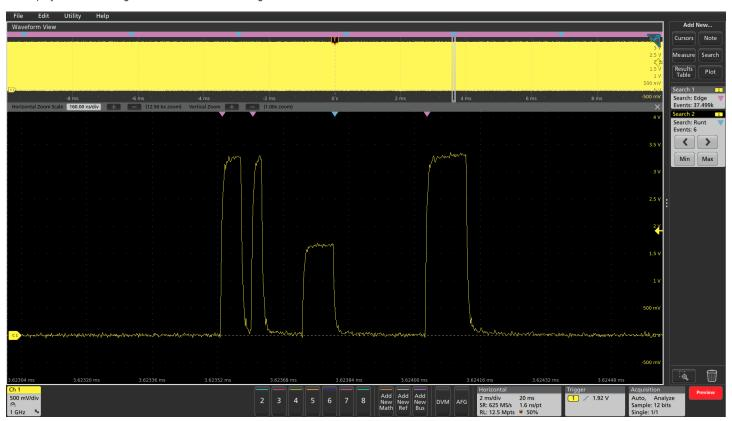
Earlier, FastAcq revealed the presence of a runt pulse in a digital data stream prompting further investigation. In this long 20 ms acquisition, Search 1 reveals that there are approximately 37,500 rising edges in the acquisition. Search 2 (run simultaneously) reveals that there are six runt pulses in the acquisition.
