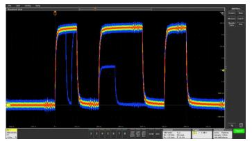
FastAcg's high waveform capture rate enables you to discover infrequent problems common in digital design.
