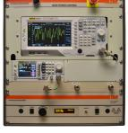
inal AR amplifier 9 kHz to 400MHz, directional coupler, and emcware® control software. Everything is contained in a single housing, which eliminates setup issues. This system provides the versatility needed for every test laboratory
