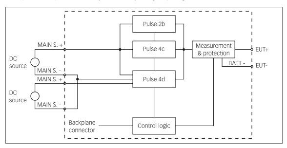
Picture 4-11: Block diagram of DS 5630 showing 2 external sources connected to it for pulse 4d
