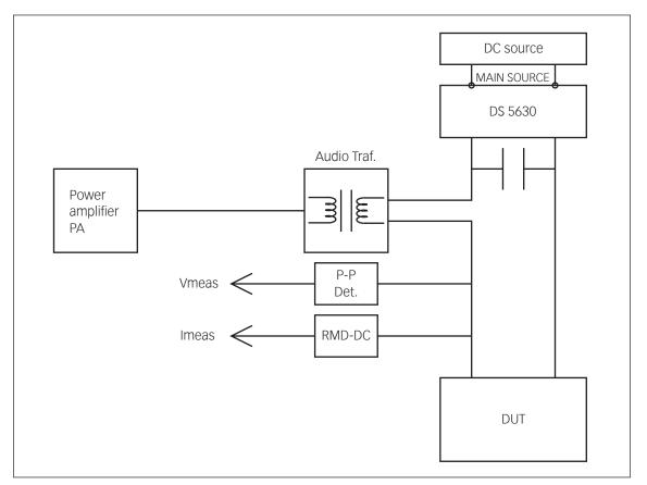
Picture 4-18: Basic block diagram of the TC 5650
