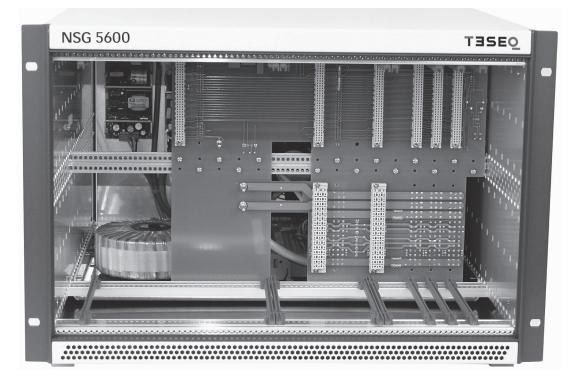
Picture 4-1: NSG 5600 system basic chassis showing the backplane and the module guide rails
