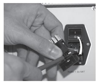
Picture 4-5: Remove defect fuses
