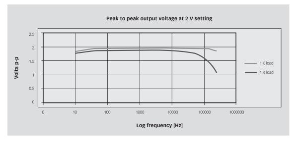
Picture 6-14: Output voltage vs frequency for a voltage setting of 2  $V_{pk\cdot pk}$  at 1  $k\Omega$  and 4  $\Omega$  loads
