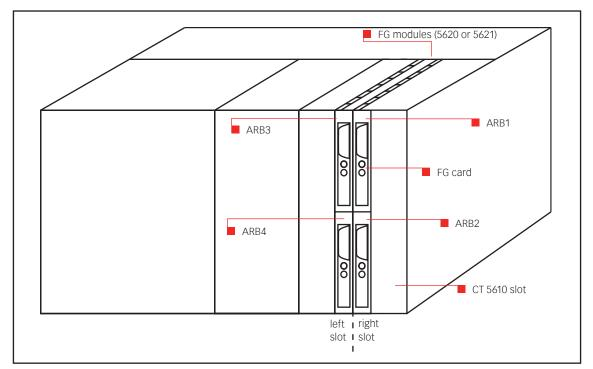
Picture 3-17: Basic chassis containing 2 FG 5621 (4 ARB cards) in left and right slots
