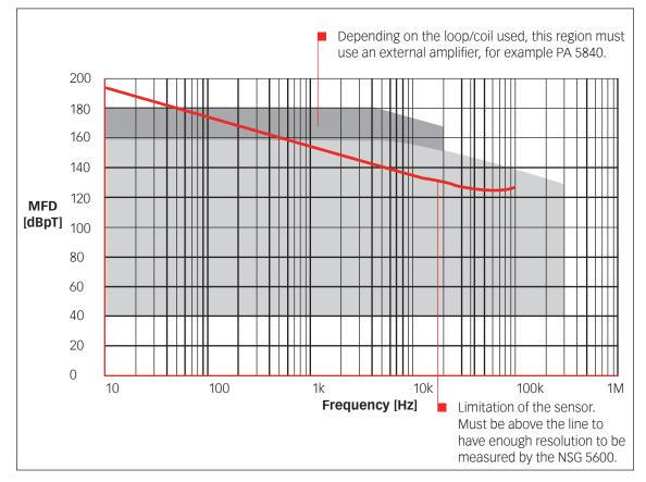
Picture 4-15: Power magnetics limitation using solar 9230-1 and loop sensor
