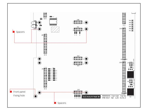
Picture 3-16: Spacer positions for the second FG card
