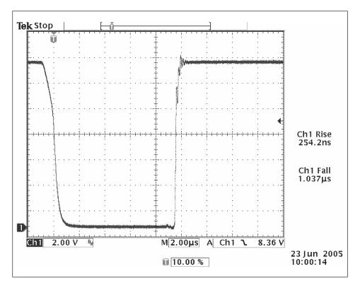
Picture 6-7: 13.5 V Dropout into 1 k $\Omega$  load for 10  $\mu s$
