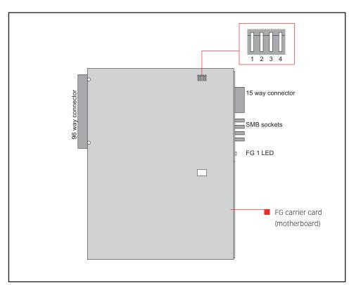
Picture 3-12: FG 5620 solder view showing the 4 way DIP switch
