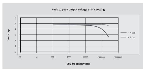
Picture 6-15: Output voltage vs frequency for a voltage setting of 5 Vpk-pk at 1  $k\Omega$  and 4  $\Omega$  loads
