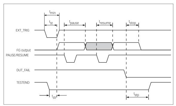
Picture 6-1: Auxiliary signals timing diagram
