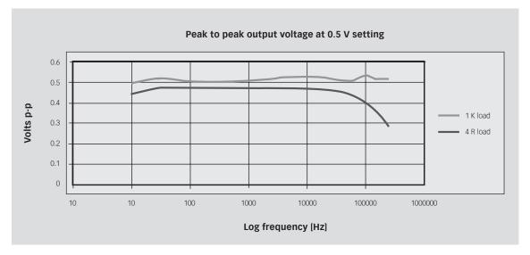
Picture 6-13: Output voltage vs frequency for a voltage setting of 0.5  $V_{_{pk\cdot pk}}$  at 1  $k\Omega$  and 4  $\Omega$  loads
