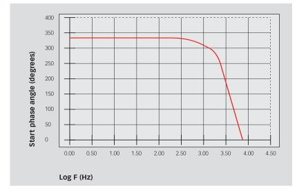
Picture 6-2: Maximum start phase angle versus frequency
