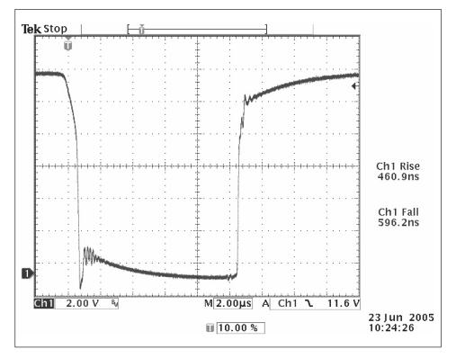
Picture 6-9: 13.5 V Dropout into 1  $\Omega$  load for 10  $\mu s$
