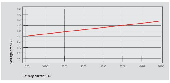
Picture 6-4: Pulse 4d Battery voltage drop vs battery current
