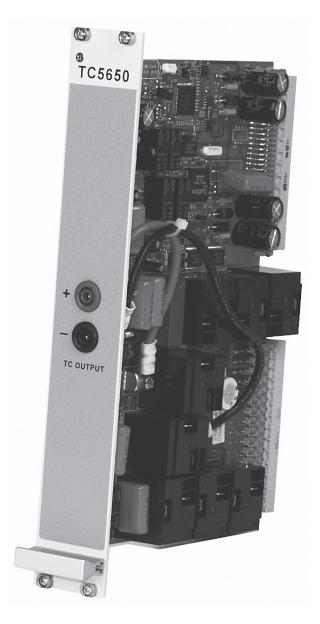
Picture 4-17: TC 5650 Conducted sine waves module
