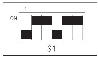
Picture 3-9: Switch S1 - GPIB address
