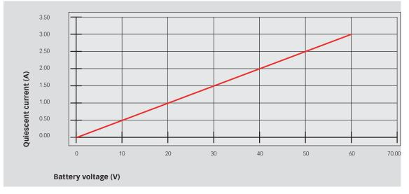
Picture 6-6: Pulse 4d quiescent current vs battery voltage
