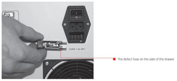
Picture 5-3: The fuses are placed on the sides of the drawer
