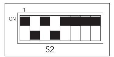
Picture 3-10: Switch S2 - CAN address
