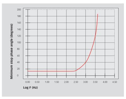
Picture 6-3: Minimum stop phase angle versus frequency
