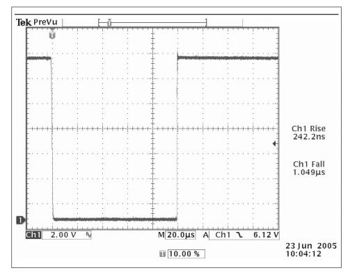
Picture 6-8: 13.5 V Dropout into 1 k $\Omega$  load for 100  $\mu s$
