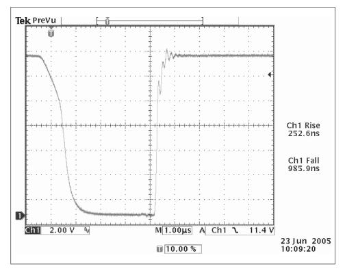
Picture 6-11: 13.5 V Dropout into 1  $k\Omega$  load for 5  $\mu s$
