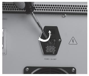
Picture 5-1: Loosen the drawer using a screwdriver
