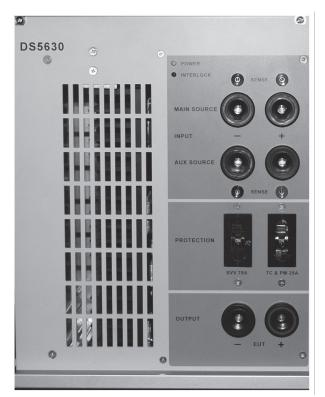
Picture 4-12: DS 5630 Front panel connectors
