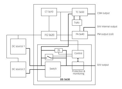
Picture 2-2: Functional block diagram of the NSG 5600 system
