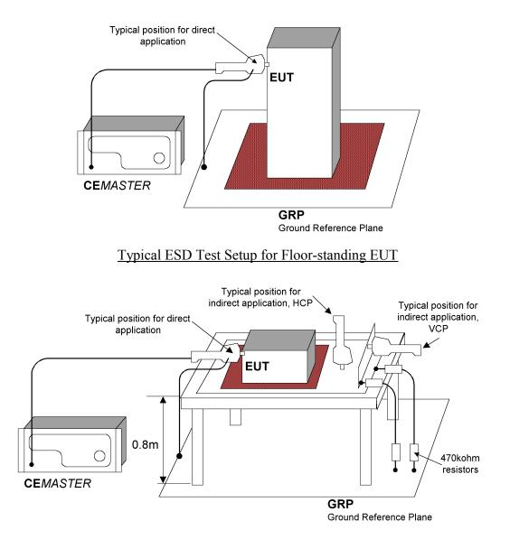
Typical ESD Test Setup for Table-Top EUT
