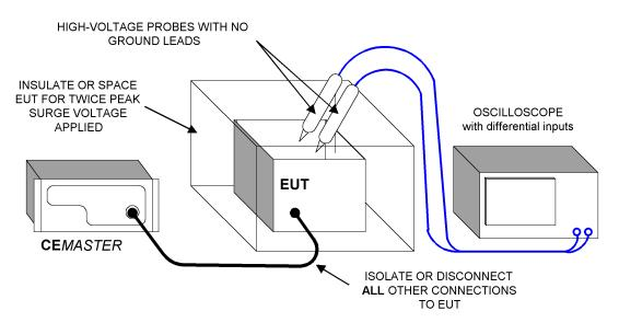
Connection of Probes to the EUT during Surge Testing
