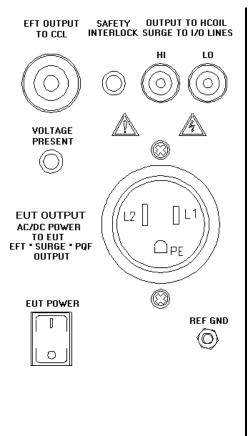
The EFT output coax, at upper left, connects to the Capacitive Cable Clamp and is used for waveform verification.
