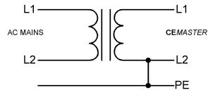
Proper Connection of an Isolation Transformer
