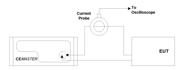
Line Qualification Test Setup -- EUT Peak Current
