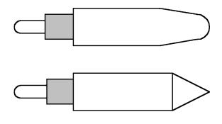
The **TPA-2** probe tip is used for air discharge. The rounded tip of this probe prevents corona (which reduces applied voltage) and ensures most consistent results.
