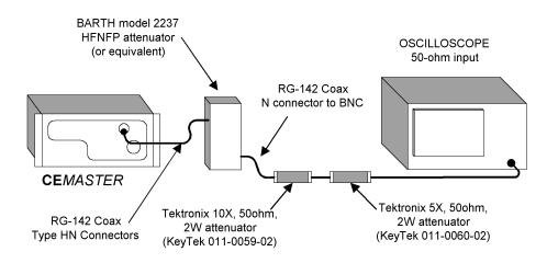
Recommended Test Setup for Waveform Verification
