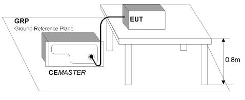
EFT Connection to Equipment Under Test for Table-top EUT
