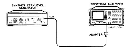
Figure 3-17. Frequency Response Test Setup (<50 MHz)
