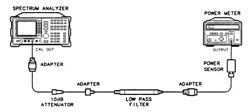
Figure 4-13. Calibrator Amplitude Accuracy Test Setup
