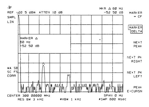
Figure 6-31. Using the FFT Function
