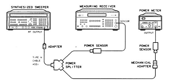
Figure 3-14. System Characterization Test Setup (Option 001)
