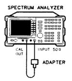
Figure 3-10. Resolution Bandwidth Switching Uncertainty Test Setup
