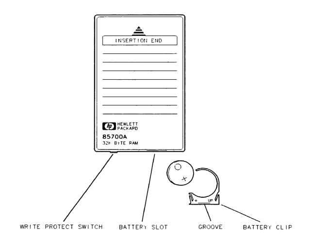
Figure 2-6. Memory Card Battery Replacement
