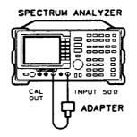
Figure 4-11. Resolution Bandwidth Switching Uncertainty Test Setup
