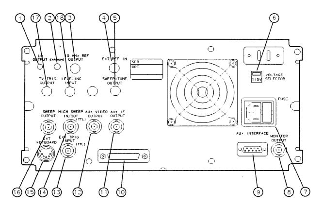
Figure 5-2. HP 8590B / HP 8592B Rear-Panel Overview
