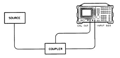
Figure 6-1. Set-Up for Obtaining Two Signals
