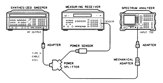
Figure 3-16. Frequency Response Test Setup, ≥50 MHz, for Option 001
