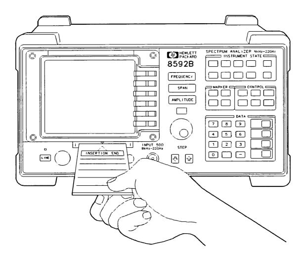
Figure 2-4. Inserting the Memory Card
