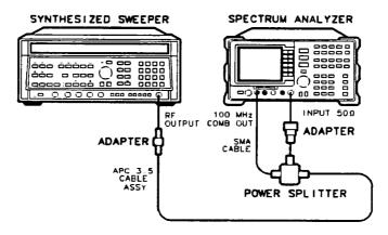
Figure 4-1. Comb Generator Frequency Accuracy Test Setup
