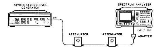
Figure 4-10. Reference Level Accuracy Test Setup
