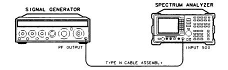
Figure 4-3. Noise Sidebands Test Setup
