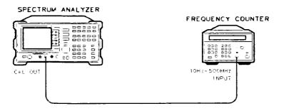
Figure 3-13. Calibrator Frequency Accuracy Test Setup
