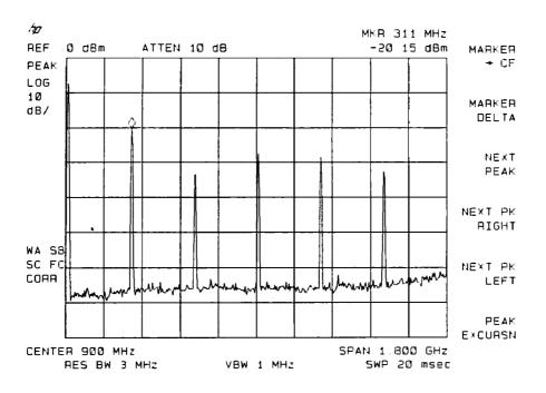
Figure 6-11. Placing a Marker on the CAL OUT Signal
