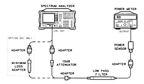
Figure 3-12. Calibrator Amplitude Accuracy Test Setup
