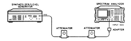
Figure 4-8. Scale Fidelity Test Setup
