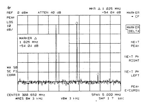
Figure 6-24. Measuring the Distortion Product
