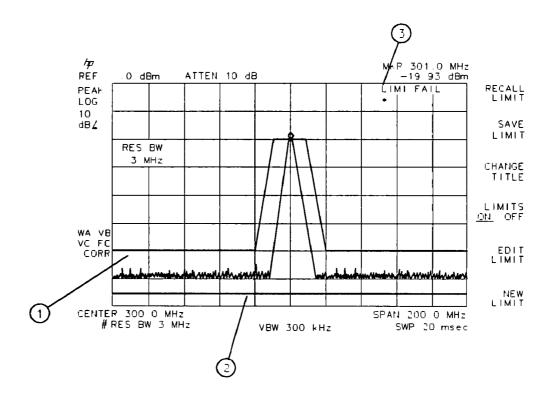
Figure 5-7. Typical Limit-Line Display
