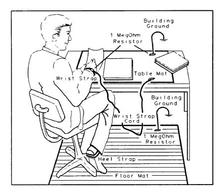
Figure 1-3. Example of a Static-Safe Work Station
