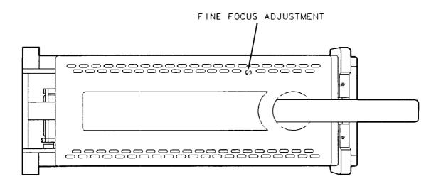
Figure 7-4. Adjusting the Fine Focus
