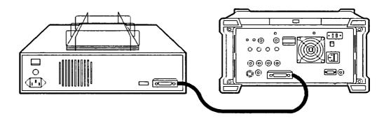
Figure 7-3. Connecting a Printer to the Analyzer
