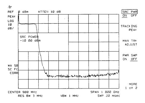
Figure 6-36. Tracking-Generator Output Power Activated
