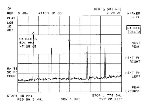
Figure 6-13. Using the Delta Meas Function
