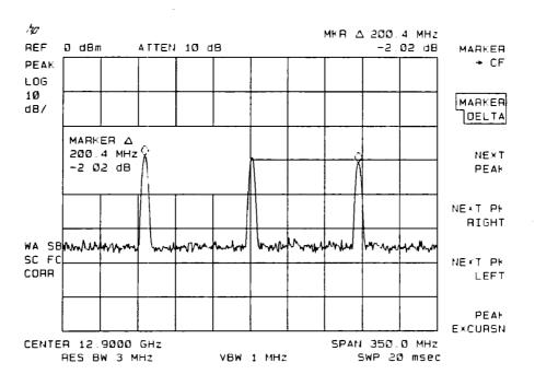
Figure 6-32. Using Harmonic Lock
