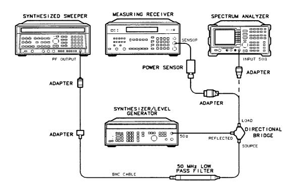
Figure 3-19. Third Order Intermodulation Distortion Test Setup
