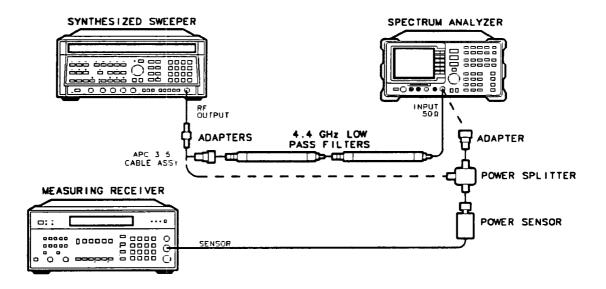
Figure 4-19. Second Harmonic Distortion Test Setup, >2.9 GHz
