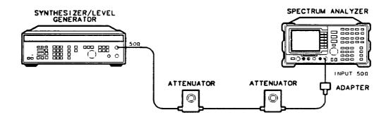
Figure 4-9. Input Attenuator Accuracy Test Setup
