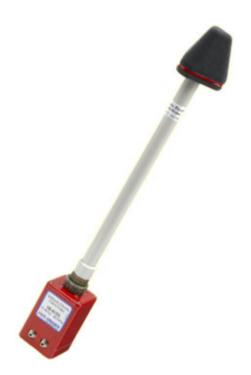
ETS-Lindgren's Model HI-6153 Laser-powered Electric Field Probes provide broadband EMF frequency coverage and wide dynamic range that satisfies the demands of most test requirements. To take advantage of this capability, the HI-6153 RF field probe was designed to be single range reading so data can be read continuously over the entire dynamic range. Data values for each axis (X,Y,Z) can be read individually, or summed.
