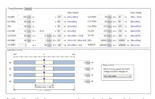
Adjusting timing parameters, including data rate, output voltage, skew rate, signal timing, and lane skew.
