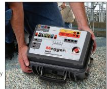
In addition the MRCT can be configured to test kneepoints up to 30 kV using an alternative DC technique. This allows testing the majority of CTs using line frequency while still being able to test larger generation class CT with a portable instrument.
