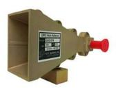
Frequency Range: 18 GHz - 40 GHz Antenna Factor: 40.3 to 41.1 Gain: 15 to 21.2 dBi Maximum Continuous Power: 10 Watts Max Radiated Field: 100 V/M Impedance: 50  $\Omega$ VSWR: 1.2:1 (1.5:1 max) Connector: 2.9mm female Mounting Base:  $\frac{1}{4}$  - 20 Thread, female
