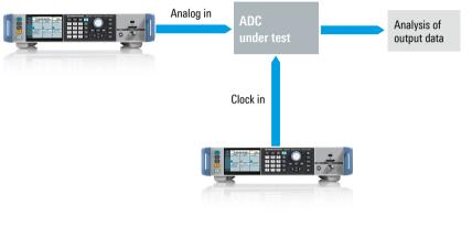
Compact ADC test setup for clock signals up to 6 GHz with a single R&S®SMA100B with an integrated second source
