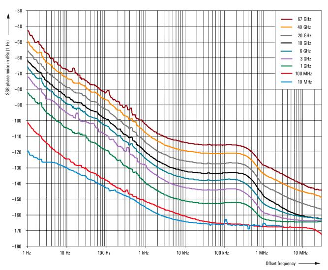
The ultimate solution is the R&S<sup>®</sup>SMAB-B711(N) ultra low phase noise option, which sets new standards with its exceptionally low phase and wideband noise across the entire offset range.
