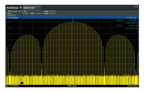
Pulse- and amplitude-modulated signal generated with the R&S<sup>®</sup>SMA100B. The sin(x)/x modulation signal is fed at the external analog modulation input and used to produce a signal with 70 dB (meas.) modulation depth
