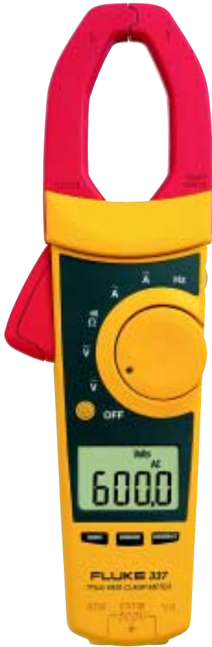
Fluke 337 The top-of-the-line True-rms clamp meter, large jaw measures ac/dc current and voltage, ohms, display hold, motor start-up current (in-rush), frequency, MIN/MAX capability and a large backlit display
