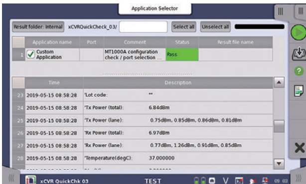
Optical Module Automatic Check Screen
