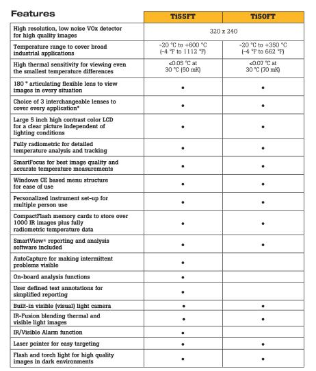
The Fluke Ti55FT and Ti50FT models feature everything needed for virtually any thermography task.
