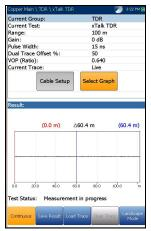
Confirmation Confirmation The XTalk test transmits the TDR pulse on the A - B pair, and receives the reflected pulse on A1 - B1 pair. The XTak test transmits the TDR pulse on the T - R pair, and receives the reflected pulse on T1 - R1 pair. onnect as per following hookup diagram : ionnect as per following hookup diagram : MAX A TX -Т T в ТΧ R R (A1) (T1 (T1) RX RX R1 R1 (B1) Cancel
