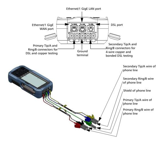
**Note:** In the MAX-63x-GVXAB model, to test an ADSL 1/2/2+ Annex B interface, the Maxtester uses the second pair (pins 2-5) in the DSL WAN RJ11 connector. When connecting the unit to a wall socket with a modem cable that uses the first pair (pins 3-4), use the red cable (pair 2) of the provided ACC-BD-RJ test cable, RJ14 to dual RJ-11, and an RJ11 female adapter ACC-RJ11-ADPTR.
