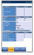
SES (severely errored seconds) (GVXAA and GVXAB models only) is the count of a one-second period that contains >30 % errored blocks or at least one severely disturbed period.
