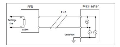
**3.** For **T-R-G/A-B-E Shorted**, connect the T-R-G/A-B-E to the customer connectors (blue-labeled Pair1- Cu) and the ground lead to the network ground.
