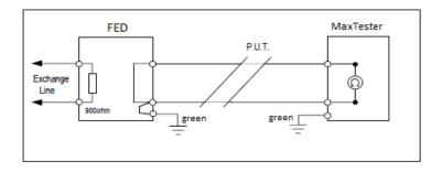
**Note:** *P.U.T.*, in the above diagrams, refers to the Pair Under Test. *Remote* is the FED, and *Controller* is the MaxTester. The **FED Control** tab displays the following parameters:
