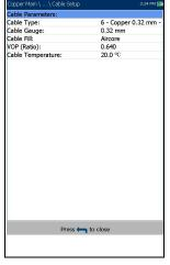
Cable Temperature is the temperature of the cable under test in either °F or °C.
