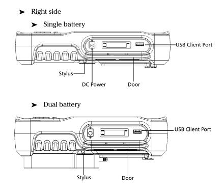
**Note:** For the dual battery, the DC power outlet is on the left side of the unit.
