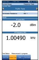
Termination Resistance lists a resistance value for the termination of the Receive Tone.
